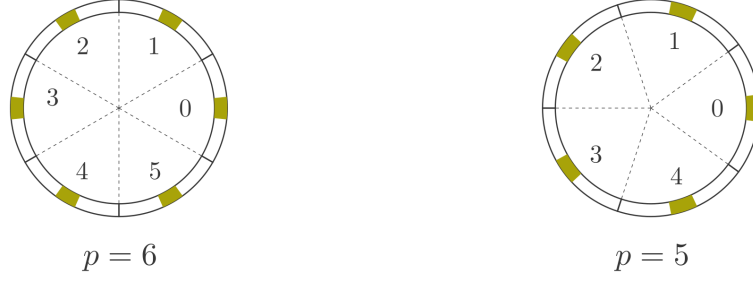
Figure 9: Distribution of the values of \mu across \mathbb{Z}_q for p = 6 and p = 5 : the colored parts show the dense spots where the value has a high probability to lie in. The width of these sectors depends on \sigma (the standard deviation of the error distribution \chi of TFHE). Note that this repartition looks the same for \tilde{\mu} in \mathbb{Z}_{2N} .
