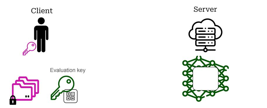
The client encrypts its data and crafts an evaluation key that will be used in the homomorphized neural network.
